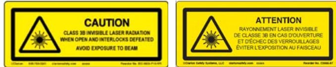
Fig 3-3. IN Cell Analyzer 2200/2000 Interlock Safety Label.
