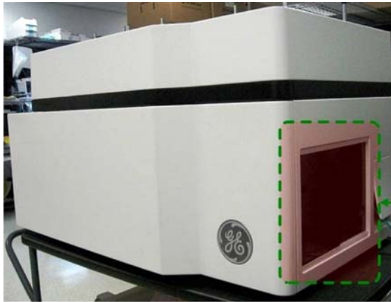
Fig 12-1. CO 2 compartment access door.
