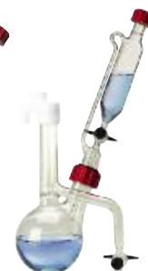
250ml Azeotropic Reaction Flask with Dropping Funnel
