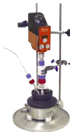
Breeze with 250ml Heat-On, stand and overhead stirrer
