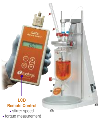
Lara includes Control Software, Data Hub and Laptop PC
