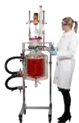
Reactor-Ready Pilot with 20 litre Vacuum Jacketed Vessel
