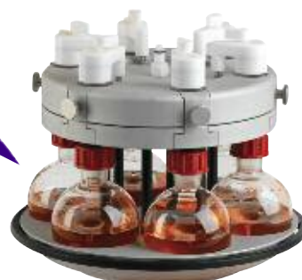
Carousel 6 locates on to the Storm without tools
