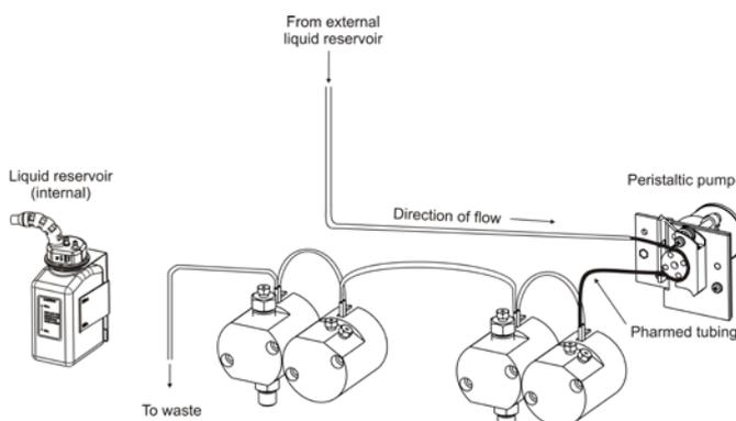
Fig. 8: Rear seal wash system (alternative setup), here for a DGP-3600
