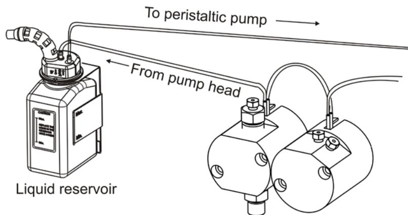
Fig. 43: Tubing connections on the internal liquid reservoir
