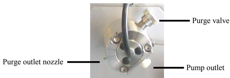
Fig. 24: Purge valve and purge outlet nozzle
