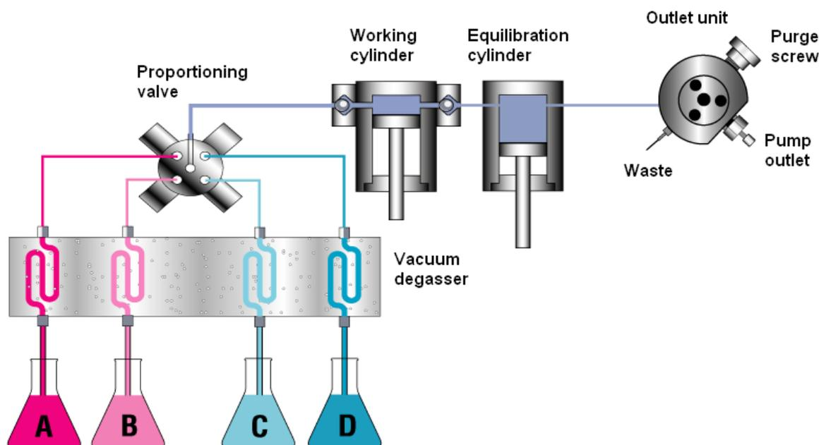
Fig. 1: LPG-3400 pump with integrated vacuum degasser
