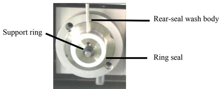
*Fig. 45: Pump head removed*
