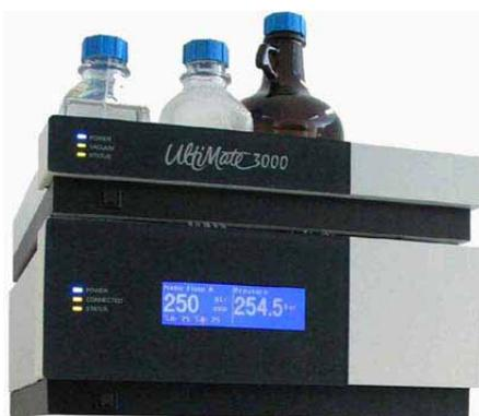
Fig. 16: Pump with Solvent Rack
