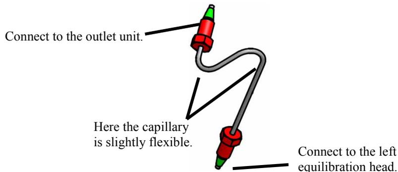
Fig. 57: Capillary from left equilibration head to outlet unit (HPG-3x00M)
