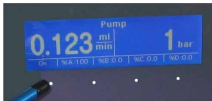
Fig. 30: Showing the function keys
