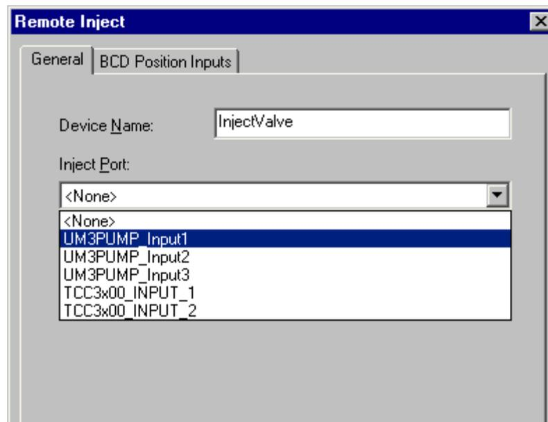
Fig. 78: Setting up the valve for external injection
