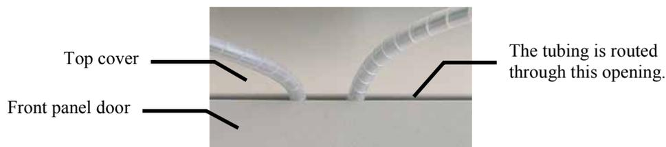
Fig. 18: Pre-connected solvent lines on a UltiMate 3000 system pump
