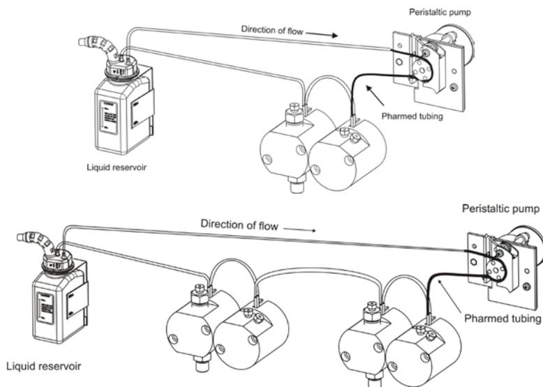
Fig. 7: Rear seal wash system (standard setup)
