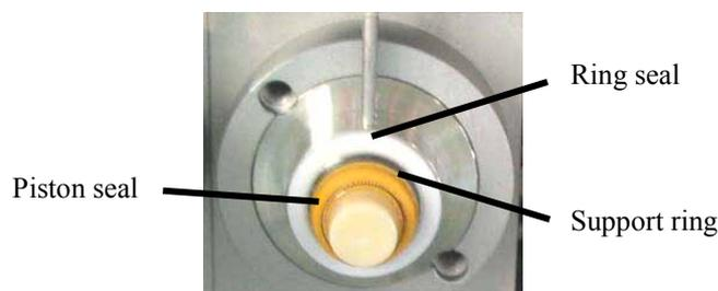
*Fig. 56: Rear seal wash system with seals and support ring*
