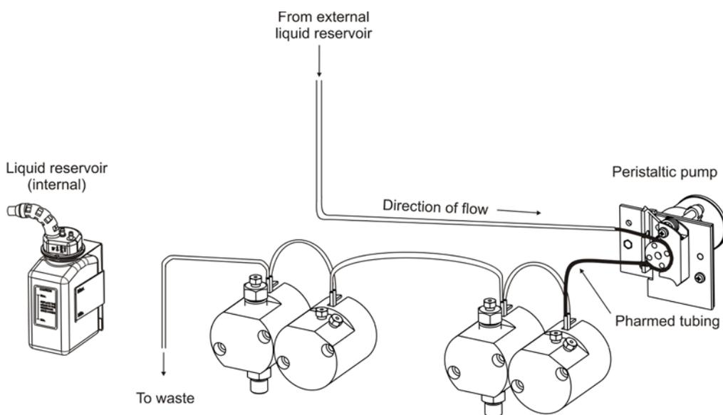
Fig. 22: Rear seal wash system with external reservoir (here for a DGP-3600)
