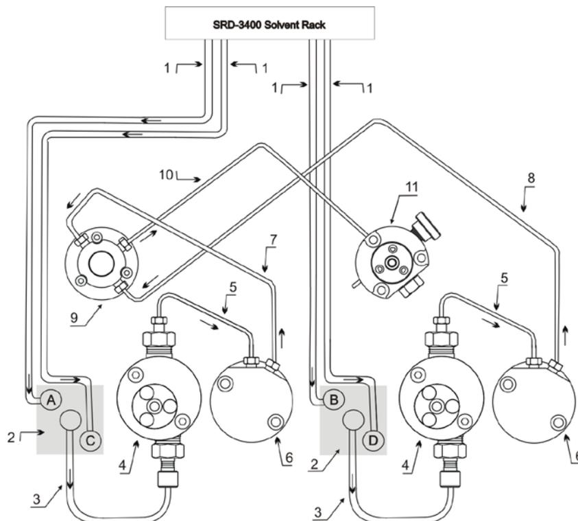
Fig. 73: Fluid connections (HPG-3400A with mixing chamber in the outlet unit)
