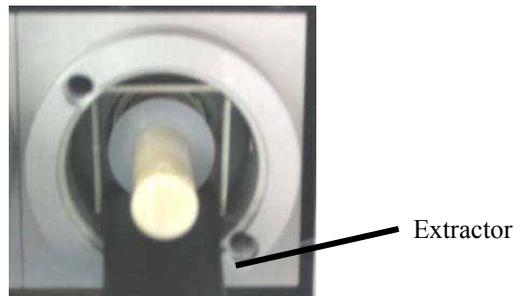
*Fig. 51: Removing the piston bushing*
