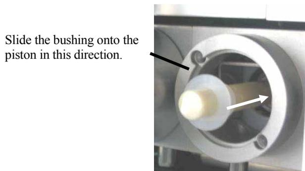
*Fig. 55: Correct orientation of the piston bushing*
