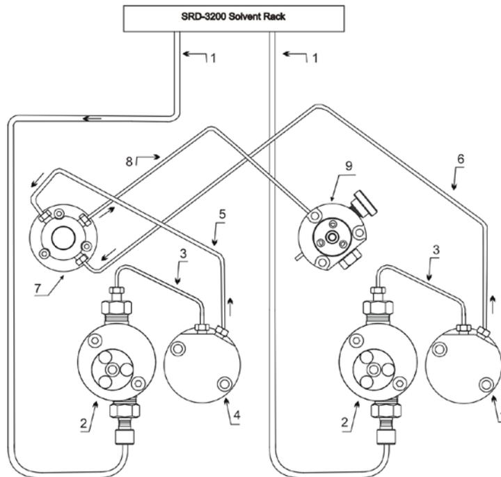
Fig. 70: Fluid connection (HPG-3200A with mixing chamber in the outlet unit)
