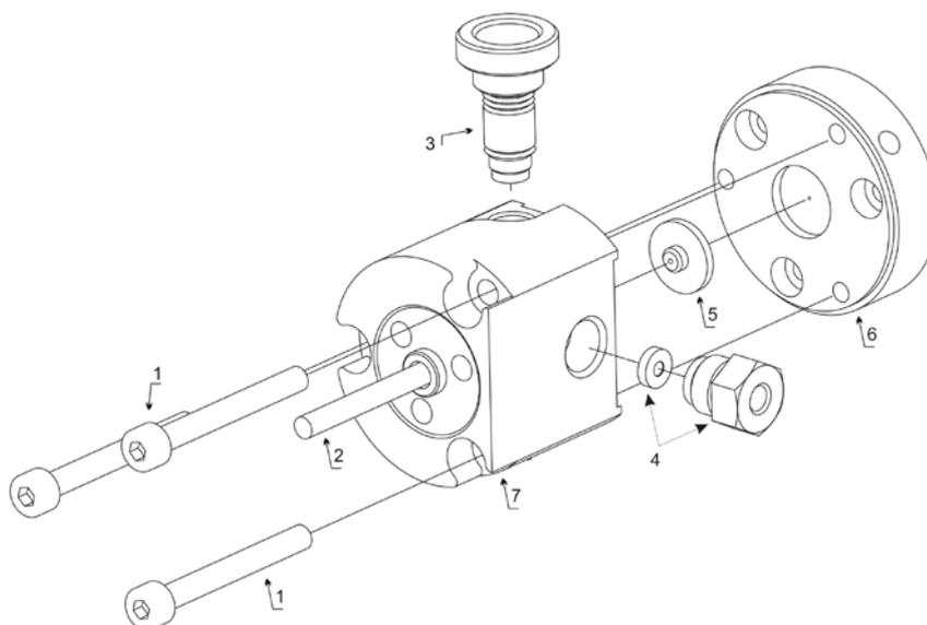
Fig. 61: Outlet unit with micro flow option
