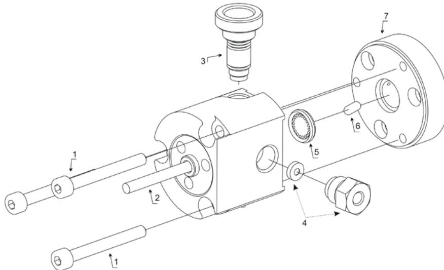
Fig. 59: Outlet unit with mixing chamber
