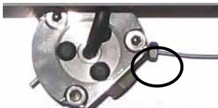
*Fig. 62: Capillaries connected to the mixing chamber base*
