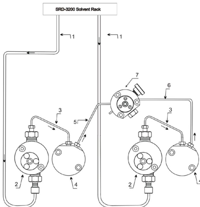
Fig. 71: Fluid connections (HPG-3200M)
