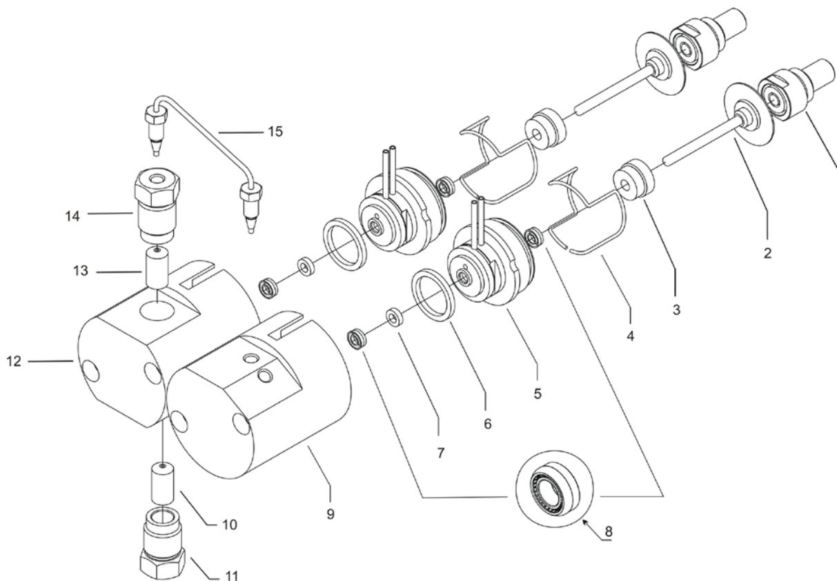
Fig. 41: Pump heads, pistons, and piston seals (here all pumps except HPG-3200P)
