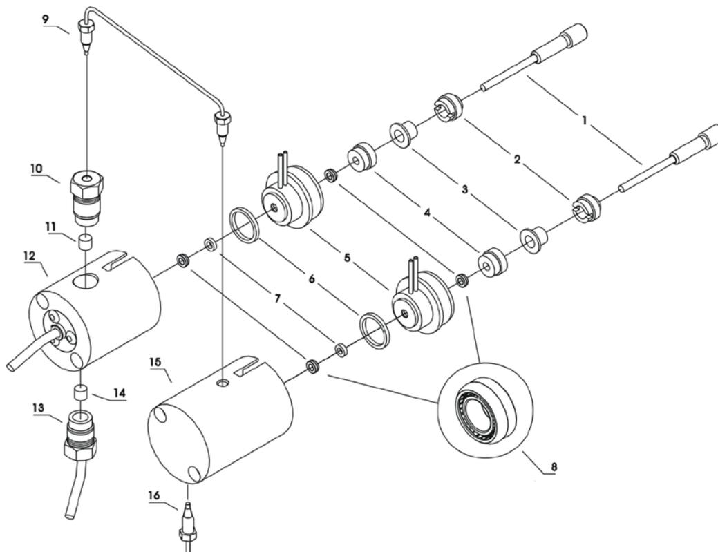
Fig. 42: Pump heads, pistons, and piston seals (here: HPG-3200P)
