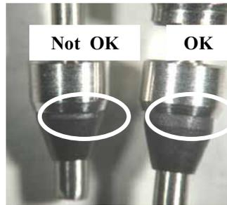
*Fig. 4: Installation of PEEK ferrules*
