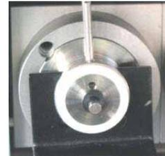
Fig. 47: Extractor on rear seal wash body
