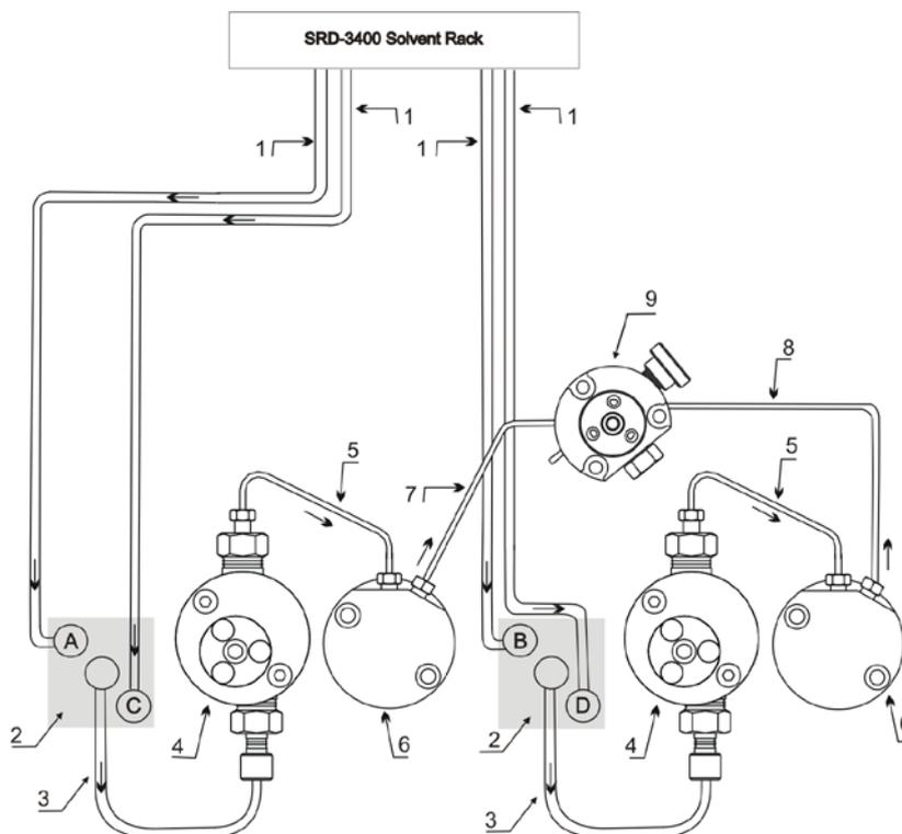
Fig. 74: Fluid connections (HPG-3400M)
