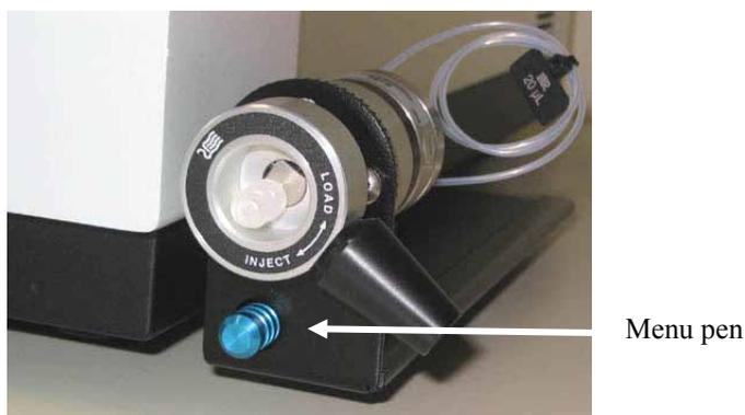
Fig. 77: Manual injection valve mounted to the pump enclosure
