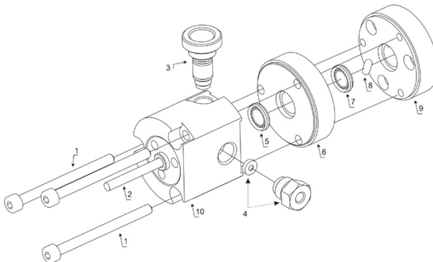
Fig. 60: Outlet unit with mixing chamber and optional extension
