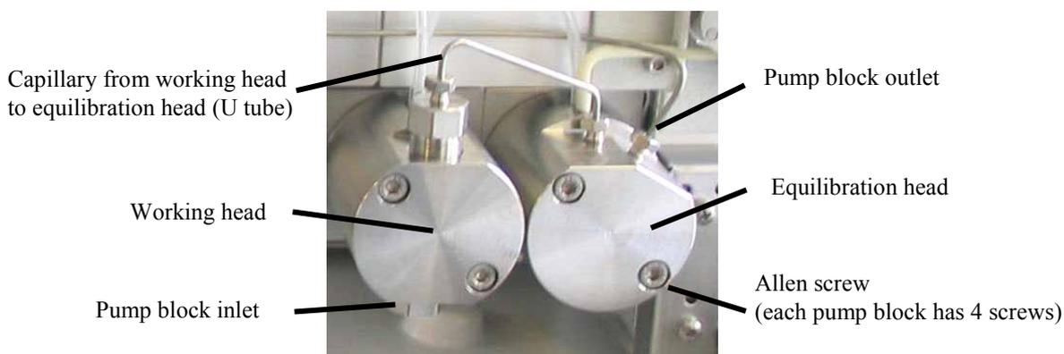
*Fig. 44: Installed pump heads*
