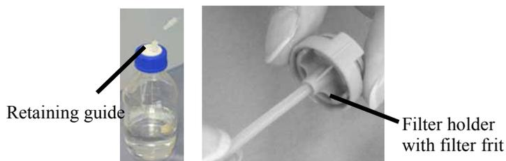
Fig. 17: Connecting the solvent lines to the reservoir
