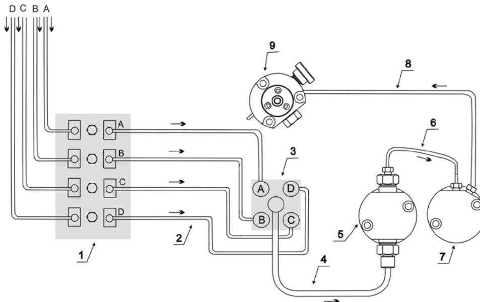
Fig. 66: Fluid connections (The arrows indicate the direction of flow.)
