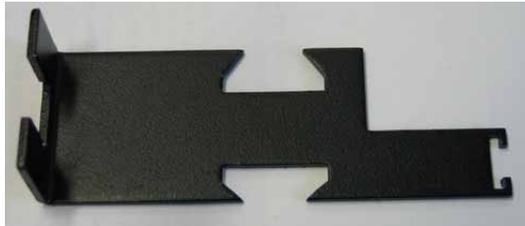
Fig. 46: Extractor for rear seal wash body
