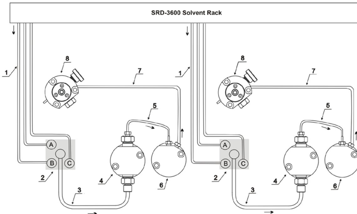
Fig. 68: Fluid connections (The arrows indicate the direction of flow.)
