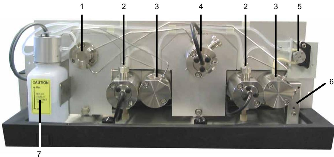
Fig. 69: Inside front panel (here: HPG-3200 with mixing chamber in the outlet unit)
