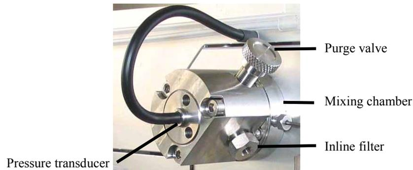
Fig. 9: Outlet unit (here with mixing chamber)
