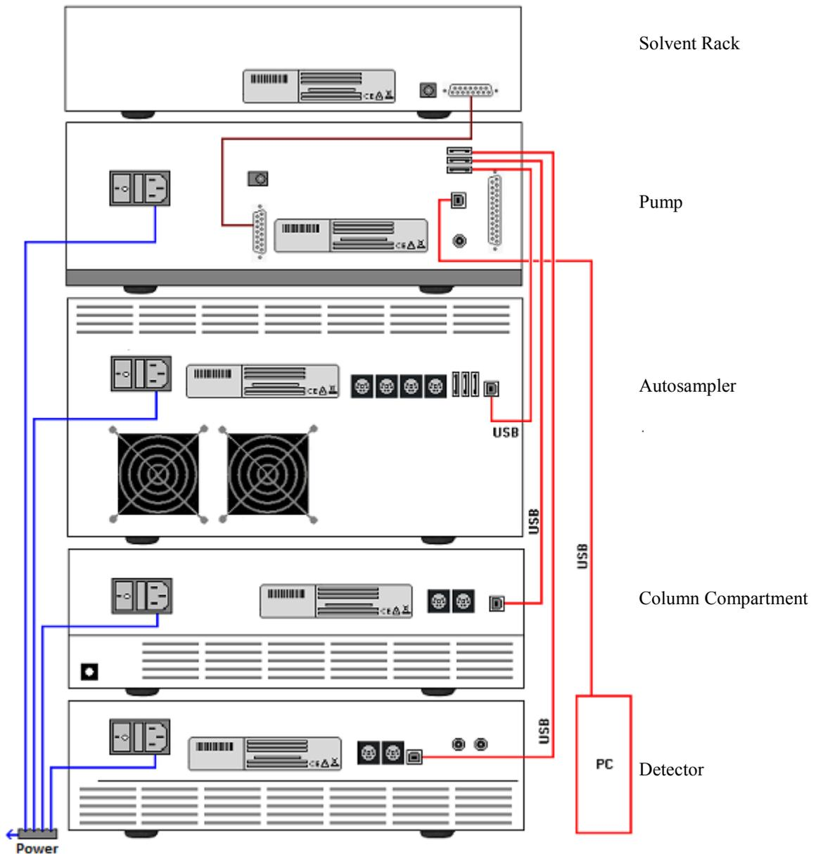
Fig. 11: Example for the rear panel connections on an UltiMate 3000 system (here with VWD-3x00)
