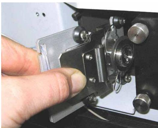
Fig. 38: Removing the flow cell
