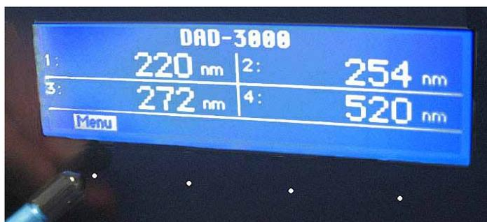
Fig. 19: Showing the function keys (here: under Chromeleon control)
