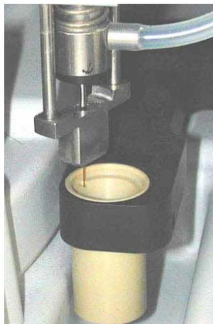
*Fig. 49: Fused silica needle in wash port*
