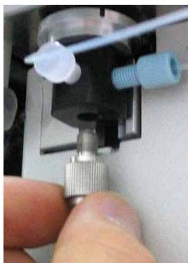
Fig. 44: Removing the syringe from the syringe valve
