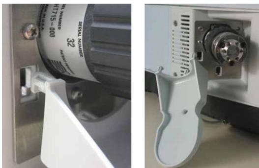
Fig. 24: Unhooking the drip tray
