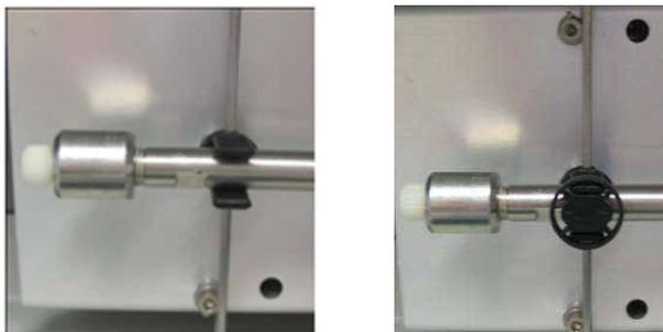
*Fig. 21: Installing a column in the clip*
