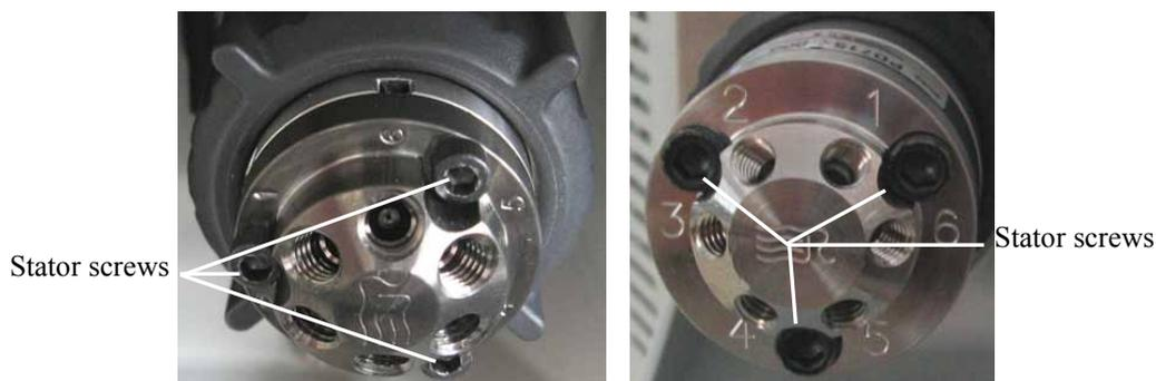
Fig. 51: Stator screws
