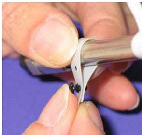
*Fig. 20: Attaching the column ID to the column*
