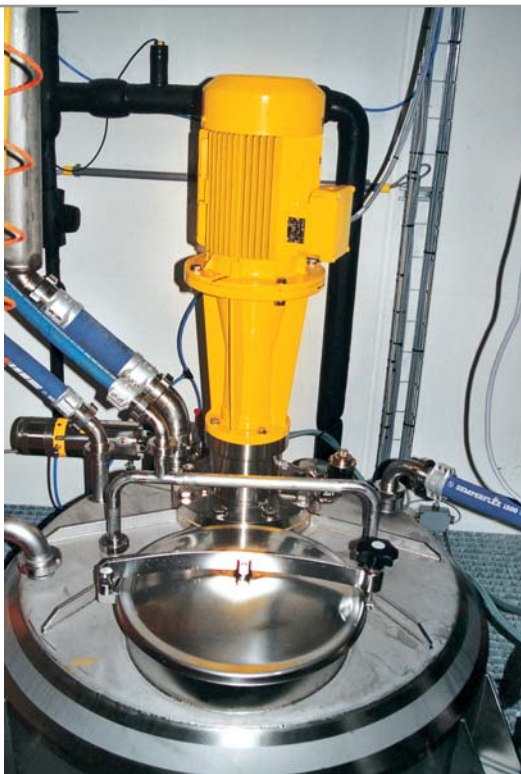
YTRON -Y HS in Tank-flange Construction Application: Suspending of Thickener Compounds
