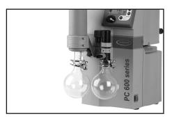
→ Assemble catchpots (9) with joint clips.
