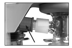
Disassemble the exhaust vapor condenser EK:
