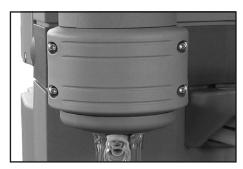
→ Remove the 4 screws affixing the counter holder of the exhaust vapor condenser with a Torx driver T10. Remove the exhaust vapor condenser. In doing so pull the PTFE hose out of the inlet of the exhaust vapor condenser.
