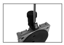
Loosen connection fastener slightly.
