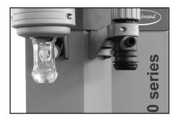
Remove catchpots (9) at inlet and outlet (see "Use and operation", page 28).
