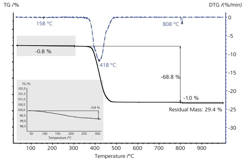
Picture-in-picture plot of the measurement on PA66/GF, heating rate of 20 K/min in a nitrogen atmosphere (40ml/min), from 800°C to 1000°C the measurement was continued in synthetic air; sample mass 10.47 mg, crucible made of alumina.
