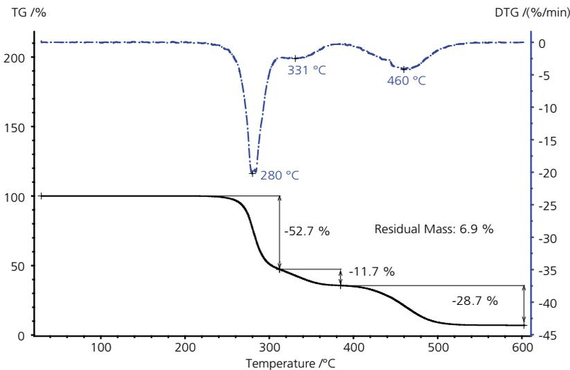
Decomposition behavior of filled PVC-U in a nitrogen atmosphere (40ml/min) at a heating rate of 10 K/min up to 600°C; sample mass 10.08 mg, crucible made of alumina
