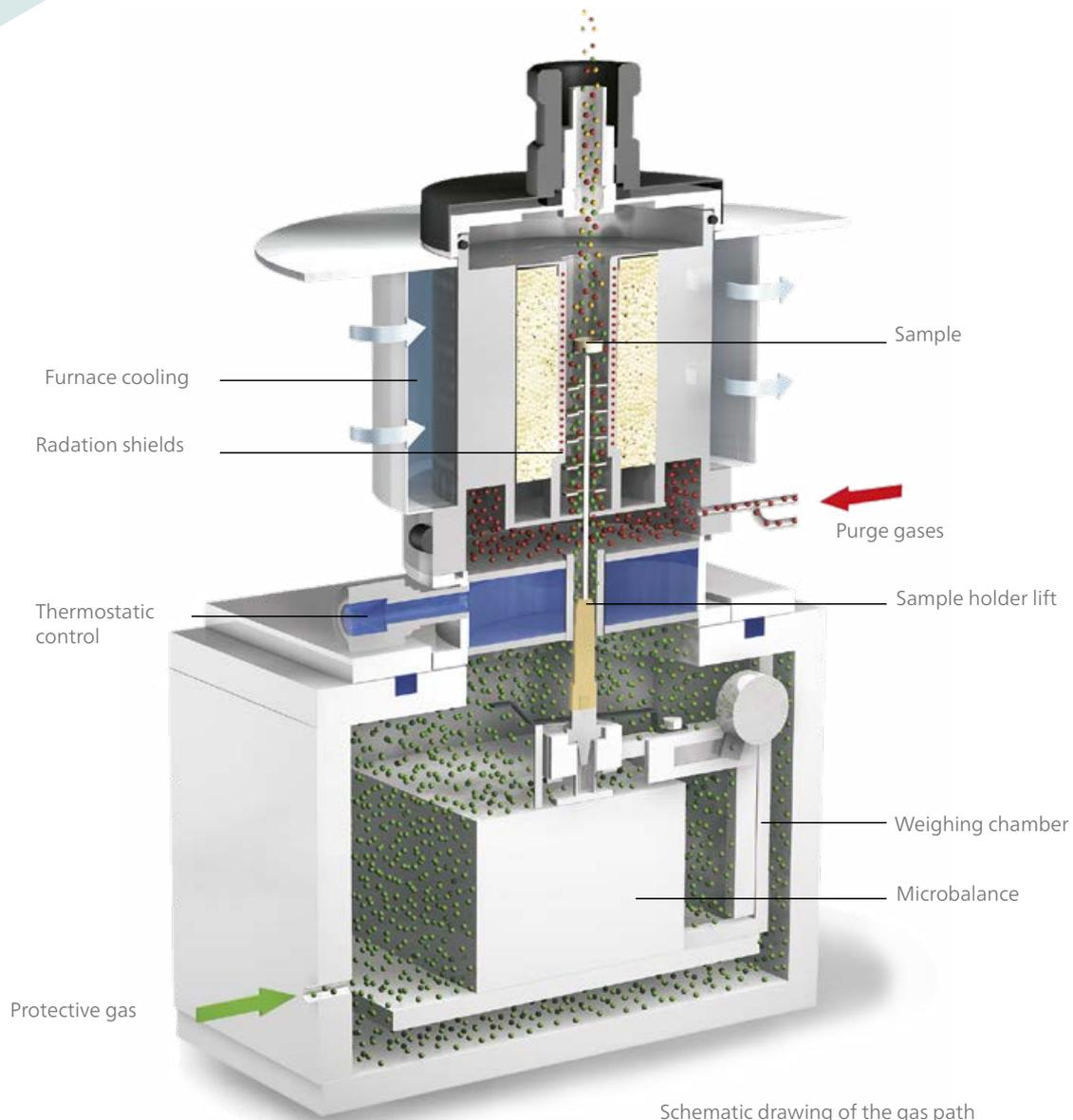
Schematic drawing of the gas path
