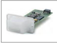
BT option: Bluetooth Interface for multipoint connection for up to 6 Bluetooth devices
