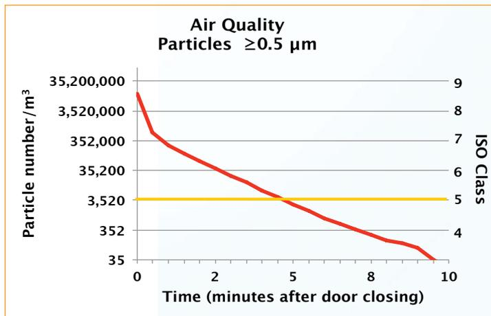
Our unique HEPA air filtration design reaches ISO Class 5 cleanroom air quality and recovers to that quality of air after a door closing within 5 minutes as tested in accordance with ISO 14644-1 and ISO 14644-3.
