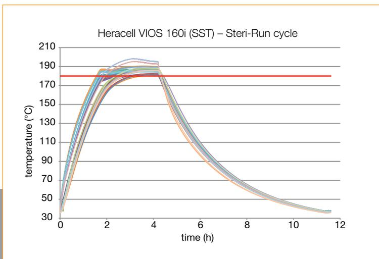
Validation that all surfaces reach 180°C with 47 point test on all chamber areas including the glass door and shelves.
