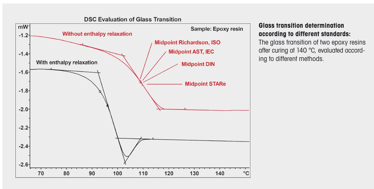
The glass transition ( $T_g$ ) can be calculated both with and without the relaxation peak according to several different standards (DIN 51007, ASTM/ICE, Richardson). You are able to choose the calculation method that suits your needs best.
