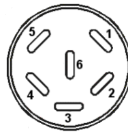
Figure 26: Zero-voltage contacts circuit diagram and pin allocation of DIN socket (9)
