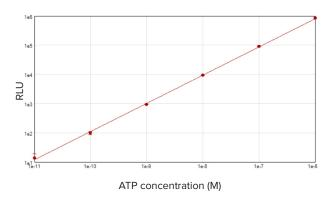
An ATP standard curve spanning five decades was run using the ATPlite 1step Luminescence Assay System (PerkinElmer) on the SpectraMax iD3 reader. Standard concentrations ranged from 1x10<sup>-11</sup> M to 1x10<sup>-6</sup> M. A wide linear dynamic range ensures accurate assay results across a broad span of sample types. Standards were plotted using a log-log curve fit in SoftMax Pro Software.
