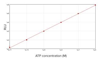
An ATP standard curve spanning five decades was run using the ATPlite 1step Luminescence Assay System (PerkinElmer) on the SpectraMax iD3 reader. Standard concentrations ranged from 1x10-11 M to 1x10-16 M. A wide linear dynamic range ensures accurate assay results across a broad span of sample types. Standards were plotted using a log-log curve fit in SoftMax Pro Software.
