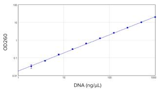
The SpectraMax iD3 reader is fully compatible with the SpectraDrop™ Micro-Volume Microplate, enabling quantitation of precious low-volume samples. 4-µL DNA standards from 2 ng/µL to 1000 ng/µL were read in absorbance detection mode with a preconfigured protocol in SoftMax Pro Software. Performance matching the 2 ng/µL sensitivity specification is demonstrated here.
