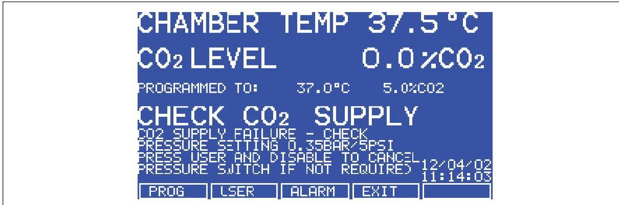
Fig. 6-10: *CHAMBER ALARM* to check CO<sub>2</sub> supply
