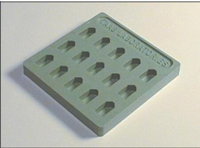
A green silicone rubber mould with 15 unmarked cavities. Specimen blocks measure 11mm x 6mm x 5mm deep, and produces a pre-trimmed trapezoidal shape at one end and a flat end at the other. Overall size of mould 68mm x 68mm.
