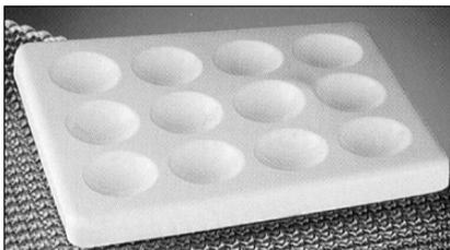
A white glazed porcelain tile, eliminates the problem associated with polypropylene tiles, that of twisting. There are 12 cavities having depression diameter of approximately 12mm and a capacity of 1ml. A high quality spotting tile for EM staining, replica washing, colour reactions etc.
