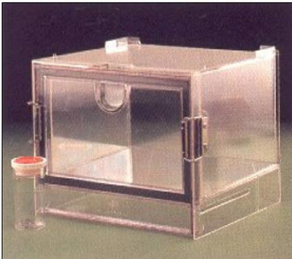
These small injection moulded high impact polystyrene cabinets are strong, rigid and airtight when closed. They are completely transparent for full visibility. The door disappears in a compartment underneath when opened. Up to 5 cabinets may be safely stacked. Supplied with a silica gel bottle. Dimensions: inside 8.25" (21cm) wide x 7" (18cm) deep x 5" (13cm) high.
