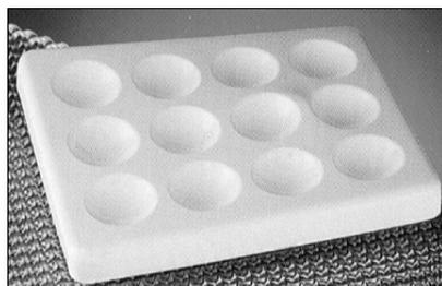
White easily cleaned tile, replacing porcelain. There are 12 cavities of approximately 1ml capacity. An economically priced, high quality, unbreakable spotting tile for EM staining, replica washing, colour reactions.
