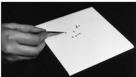
Provides a background of good visibility for handling specimens which are not normally easily seen, for trimming specimens to a size suitable for processing. Easily kept clean, white ceramic 150mm x 150mm.
