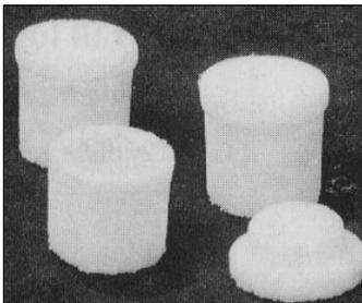
These solvent resistant small porous capsules with push-on lids can be used for many processing applications for fragile specimens. The microporous structure allows liquid exchange but the walls retain sufficient reagent to keep specimens moist up to the dehydration stage. The capsules are extremely useful for safely containing biological specimens during processing for Critical Point Drying. Also useful for specimen desiccation procedures. Average pore size 80µm
