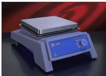
**SB160** (was SH1) Rugged and reliable hotplate with 16 x 16cm cast aluminium/silicon alloy top which will easily withstand the knocks of everyday use. The cast aluminium body is shaped for stability and also helps deflect spills away from the controls and the user. Fitting for detachable retort stand situated on the back of the instrument.
