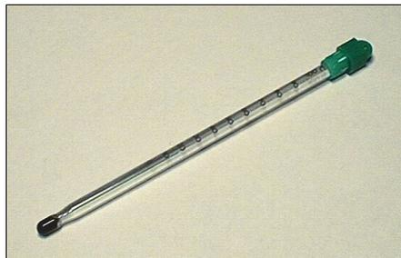
A short form robust *total immersion* stirring thermometer, with a **reinforced bulb**. The thermometer is only 150mm long and will stand in an empty 50ml beaker without causing it to fall over. Calibrated in degrees Celsius on white background, with a range of  $-10$  to  $110^{\circ}\text{C}$ .
