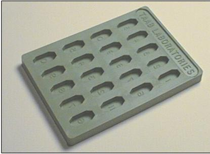
This green silicone rubber mould will produce pre-trimmed trapezoidal flat blocks shaped at both ends. Capacity 20 numbered cavities, the block size produced is 14mm x 6mm x 4mm deep. Overall size of mould is 93 x 62mm.
