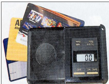
A pocket balance in credit-card format. The draughtguard over the weighing area and display, protects the balance and also serves as a weighing pan.
