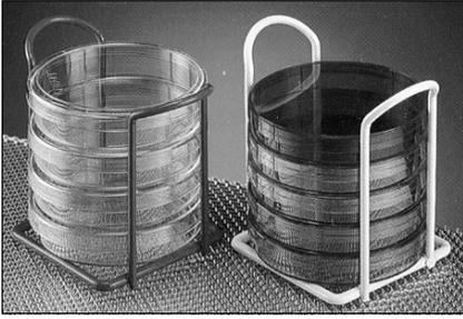
These useful stands will hold up to six 90mm Petri dishes. Manufactured from epoxy coated steel, dispenses 90mm Petri dishes from the base by gravity feed. Fully autoclavable and ideal for small batch incubation. The stands are available in seven different colours for easy batch coding.
