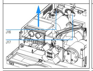
**7** Place the new pump drive into the recess in the foam part and connect the cables to the connectors on the main board (J16 Motor, J17 Encoder).
