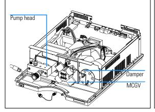
1 Remove the pump from the stack, remove the front cover, top cover and top foam section (see "Removing the Top Cover and Foam" on page 128).
