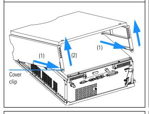
**4** Unscrew the screws on the top plate and remove the plate by lifting its back first and then sliding to the front.
