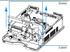
4 Disconnect the connectors of the pump assembly (J16, J17), fan (J25) and damper (J24) at the main board and lift the three assemblies out of the foam. Disconnect all remaining connectors at the main board.
