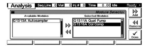
Here, e.g. the autosampler and thermostatted column compartement parameters are shown on the display as well. The number of parameters on the display is restricted as additional modules are added. A maximum of 4 modules is shown automatically. If more modules are connected to the system, you have to choose 4 of them in Setup view.
