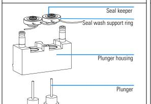
**3** Using the blade of a flat-blade screwdriver remove the seal wash gasket and the secondary seal from the support ring.
