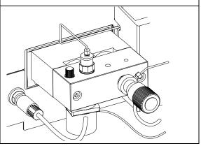
3 Clean the pump chambers, ensure all particulate matter is removed. Best cleaning results will be achieved by removing all three valves (see pages 103, 106 and 108) and injecting solvent into each chamber.
