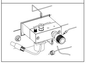
**2** Using a 4-mm hexagonal key stepwise loosen and remove the two pump head screws and remove the pump head from the pump drive.
