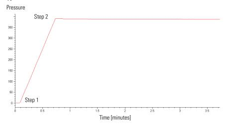
Step 1 The test begins with the initialization of the pump. After initialization, plunger 1 is at the top of its stroke. Next, the pump begins pumping solvent
