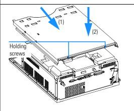
**6** Replace the top cover. Replace the pump on stack, reconnect all tubings and cables.
