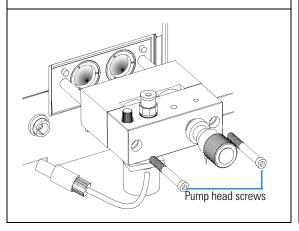
3 Place the pump head on a flat surface. Loosen the lock screw (two revolutions) and while holding the lower half of the assembly carefully pull the pump head away from the plunger housing.
