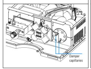
**4** Loosen the screws of the Z-panel and take it out of the instrument.
