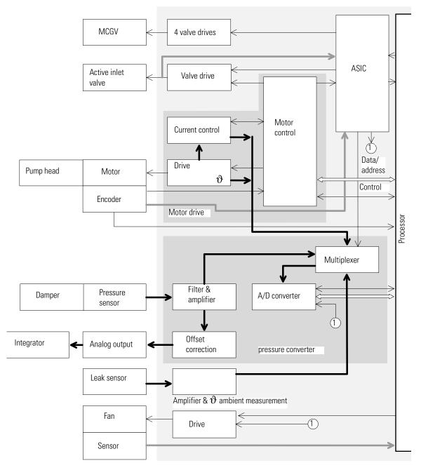
Figure 46 Interconnection Diagram Low Pressure Main Board (LPM)
