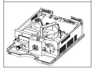
17 Install foam and top cover, see "Replacing the Top Cover and Foam" on page 156. Replace the pump on stack, reconnect all tubings and cables.
