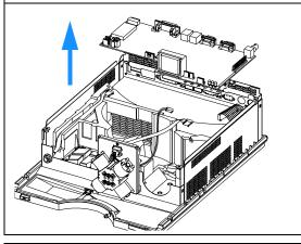
**6** Push the leak sensor cable through the recess in the foam and lift the bottom foam out of the instrument.
