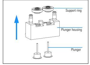
**5** Check the plunger surface and remove any deposits or layers. Cleaning can be done with alcohol or tooth paste. Replace plunger if scratched.
