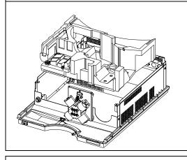
13 Reinstall the main board, see "Exchanging the Low Pressure Pump Main Board (LPM Board)" on page 131.
