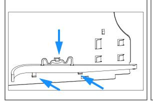
**2** Replace the top cover, see "Replacing the Top Cover and Foam" on page 156.
