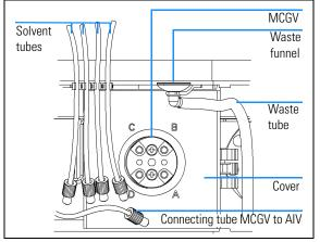
**2** Press the lower sides of the cover to unclip it. Remove the cover.
