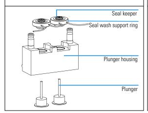
**7** If necessary replace the pump seals (see page 112). Reassemble the pump head (see page 121).
