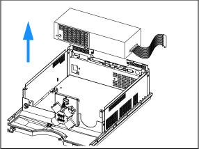
10 Place the new power supply into the instrument and fix the two screws at the back plane.
