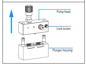
**4** Remove the support rings from the plunger housing and lift the housing away from the plungers.
