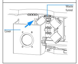
6 Reconnect the tube from the active inlet valve to the middle position of the MCGV and then the solvent tubes at channel A to D of the MCGV. Make sure the orientation of the channels on the cover is labelled as shown below, otherwhise re-label the cover.
