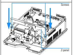
16 Clip the MCGV cover into position. Reconnect all capillaries, tubes and cables to the pump head, the MCGV and the damper.
