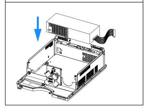
11 Install the coupler onto the power supply switch and clip the light pipe back onto the coupler.
