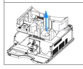
**7** Loosen and remove the power supply screws at the rear panel.
