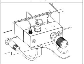
2 Remove the seal keeper and the seal wash support rings from the plunger housing. Remove the seal keeper from the support ring assembly.
