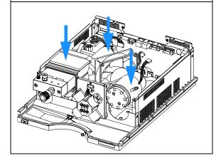
**15** Place the Z-panel into its position and tighten the two screws.
