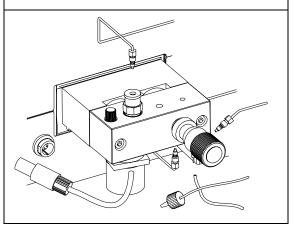
4 Loosen the screws of the Z-panel and take it out of the instrument.
