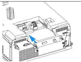
5 Replace the metal cover (slide the metal tabs into place (1) underneath the Z-Panel in the front, then lower the back of the metal plate (2)) and fix the two holding screws.
