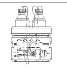
**9** Replace the leak funnel with the waste tube. Locate the lower end of the waste tube in the holder of the leak pan and clip tube to the holder at the gradient valve cover.
