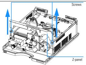
**5** Disconnect the damper connector at the main board (J24). Lift the damper out of its position.
