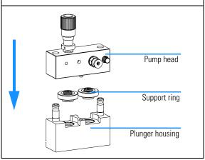
2 Insert the plungers and carefully press them into the seal.
