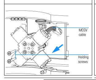
4 Place the new MCGV into position. Make sure that the valve is positioned with the A-channel at the bottom-right position. Tighten the two holding screws and connect the cable to its connector.
