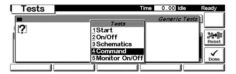
Enter 'TYPE G1311A' in the Instr-line in order to configure the module as a quaternary pump.
