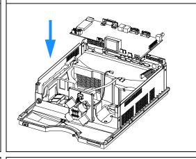
14 Re-install pump assembly, fan and damper into the bottom foam and re-connect to the main board.
