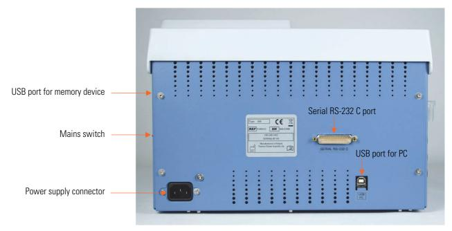
Figure 3–25. Wellwash Versa back view
