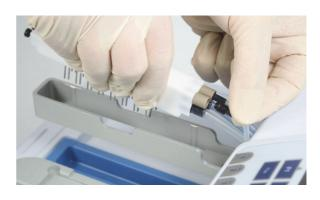
Figure 2–14. Installing the 2x8 cell wash head onto the wash head arm
