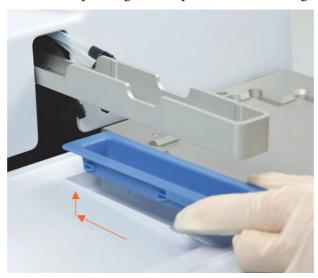
Figure 11–42. Removing the priming vessel
