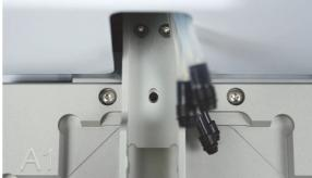
Figure 11–47. Aligning the plate carrier and wash head arm
