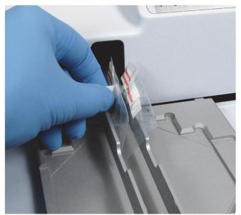
Figure 2–6. Transport lock and transport lock tag
