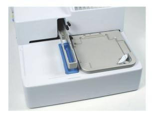
Figure 2–8. Priming vessel installation
