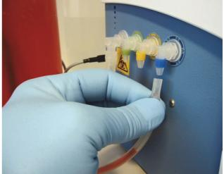
Figure 11–46. Manually priming a dry pump. Colored liquids are used for illustrative purposes.
