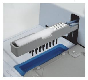
Figure 2–12. 2x8 wash heads evenly inserted
