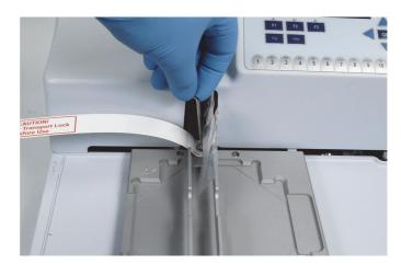
Figure 11–48. Fastening the transport lock
