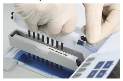
**Figure 2–10.** Fitting the wash heads to the connectors
