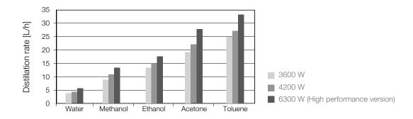
The maximum achievable distillation rate depends is not just related to the heating capacity, but also on rotation speed, flask size and temperature difference between bath and cooling.
