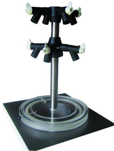
1. The manifold is connected to the conus in the lid. Make sure this connection is tight. Check that all rubber valves are closed **(A)** or in vacuum-release position **(C)**, and that the flange and lid are tight.
