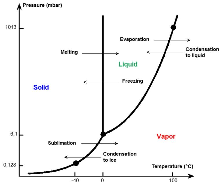
As shown in the diagram for water, the physical state is dependent on the surrounding pressure and the temperature. The point where all three phases of water co-exist is called the triple point.
