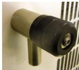
A hose may be attached to the nozzle to minimize spillage. Remember to close the drain valve after use.
