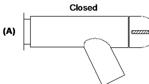
2. Start the creation of vacuum by opening the vacuum valve and check that the AWO-Indicator stays green indicating OK for freeze-drying.
