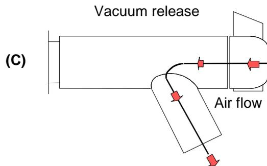
5. Close the vacuum valve after removal of the last flask.
