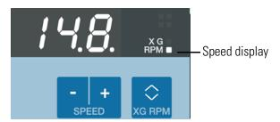
2. When the upper indicator is lit the display shows the RCF value. Press the key to toggle between the two modes.
