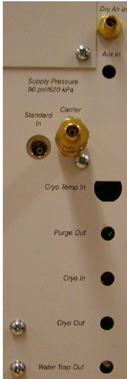
**Figure 20 Connections on back of the instrument**
