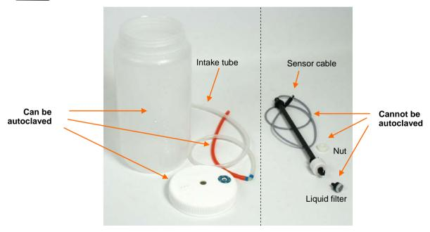
Figure 38. Autoclavable and un-autoclavable liquid bottle parts
