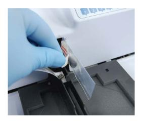
Figure 5. Transport lock and transport lock tag
