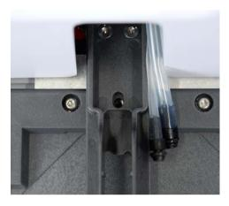
Figure 41. Aligning the plate carrier and wash head arm
