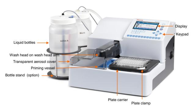
Figure 21. Wellwash front view with accessories
