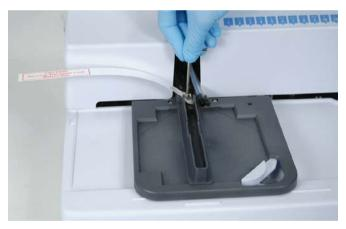
Figure 42. Fastening the transport lock
