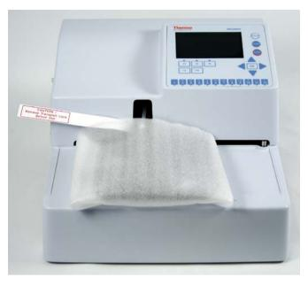
Figure 43. Transport lock and tag fitted
