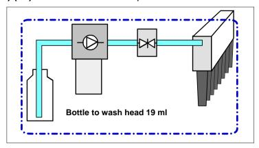
Figure 30. Dead volume of the liquid tubing
