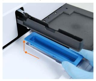
Figure 36. Removing the priming vessel
