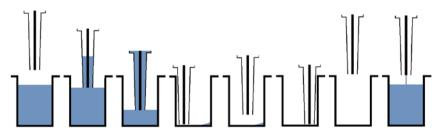
Figure 4. Principle of Wash step (Sweep2)
