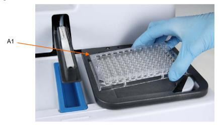
Figure 29. Inserting the microplate in landscape mode
