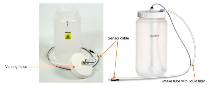
Figure 12. Waste and liquid bottles with liquid level sensors
