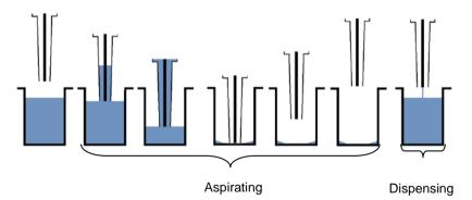
Figure 32. Principle of Wash step (Normal)
