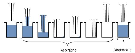
Figure 33. Principle of Wash step (Sweep2)
