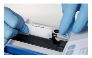
Figure 9. Fitting the wash head to the connectors
