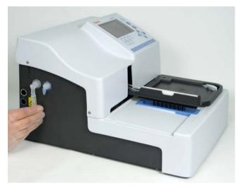
Figure 15. Connecting the liquid bottle tubing
