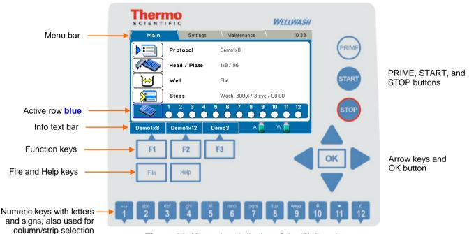
Figure 26. Keypad and display of the Wellwash
