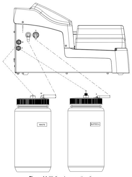
Figure 14. Wellwash connection diagram
