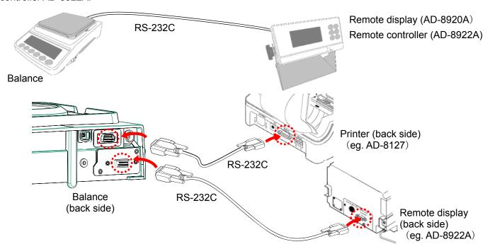
It is also possible to connect a printer to a remote controller (AD-8922A). For details, please refer to the AD-8922A instruction manual.
