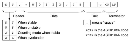
☐ The external key print mode of the AD-8127 multi-function printer is as follows when the A&D standard format is received.:
