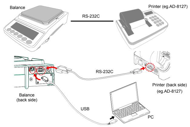
If only the balance is connected to the PC, it can also be connected using a USB cable or RS-232C cable.
