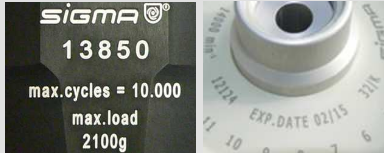
Fig. 3.1: Different service life – engraving on the bucket/rotor
