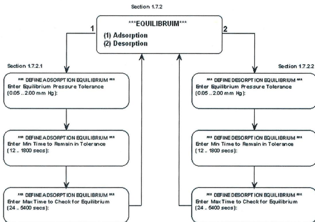
When the time tolerance has been entered, the display will prompt you to enter a maximum time to check for equilibrium. This dwell time is a "time out" value which determines when a data point will be accepted if the pressure does not reach equilibrium and does not fall out of the pressure limit range. The acceptable time range is from twice the equilibration time to 5400 seconds.
