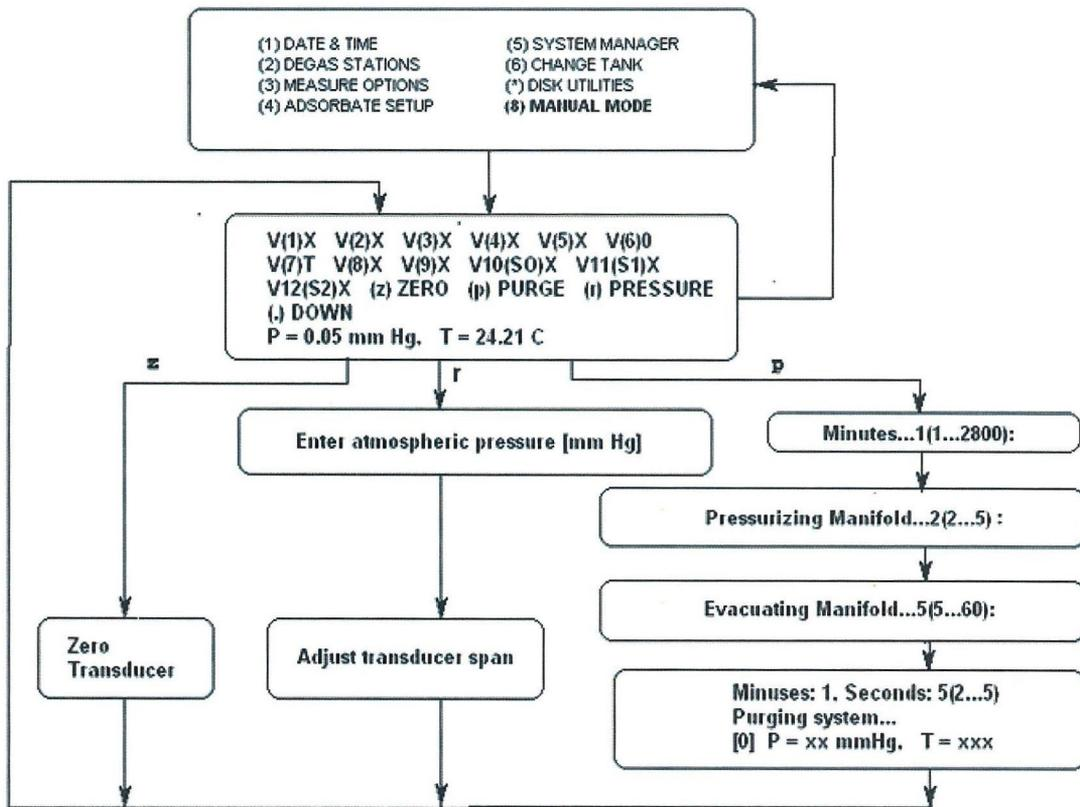
**Note:** Only experienced NOVA users should access this option. Access to MANUAL MODE can be locked out using the SYSTEM MANAGER lockouts.
