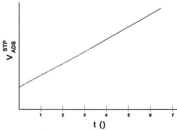
Fig. IV. t-plot of a microporous sample.
