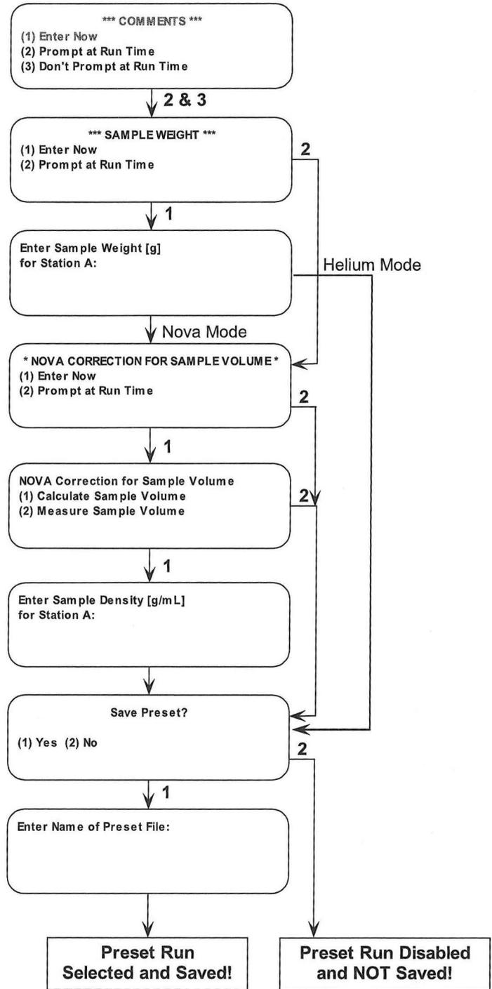
7. Next, if your NOVA is currently in the Helium Mode (model 26 only), you will go directly to the – final step. However, if your instrument is in the Nova Mode, first you will be asked to choose option for the **NOVA Correction for Sample Volume**. You can: (1) Enter the correction now, or (2) be prompted to do so at Run Time. The correction is based on (1) calculation of a sample volume, in which case you must input sample density (in g/mL) or (2) measurement of a sample volume at Run Time.
