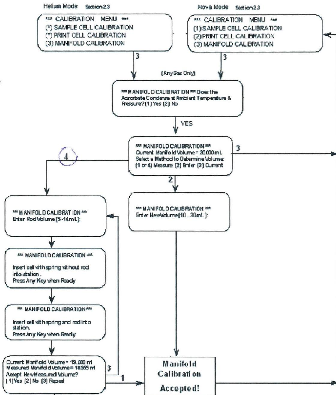
The LCD panel then displays the values of the current manifold volume and the new measured volume. Select either one as required or press (3) to measure the volume again.
