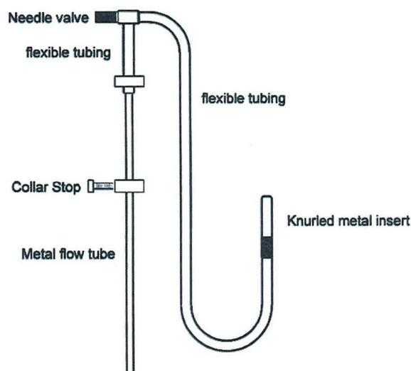
**Figure 1: Flow Degasser Assembly**
