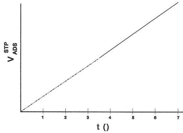
Fig. III. t-plot of a mesoporous material.
