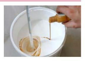
Paint, ink and adhesives are demanding applications that require an overhead stirrer that can deliver maximum torque. The Achiever 200 with the Turbine stirring shaft can mix samples with medium to high viscosity at all speeds and handle a capacity up to 100L. The Turbine stirring shaft's unique shape creates a vortex in the sample through radial flow for thorough mixing. The Telescopic-H Support Stand allows for quick and easy positioning of the stirring shaft in the sample.
