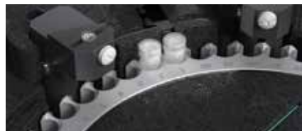
Autosampler carousel with vial sensor and inlet/outlet lifts
