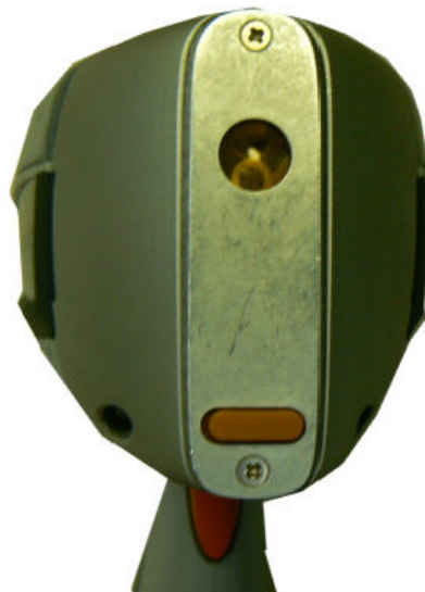
Figure 6. View of Face Plate and measurement window
