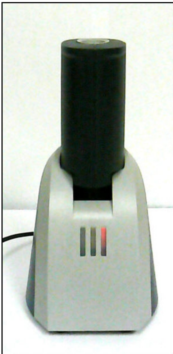
Figure 13. Battery Pack in the Charger
