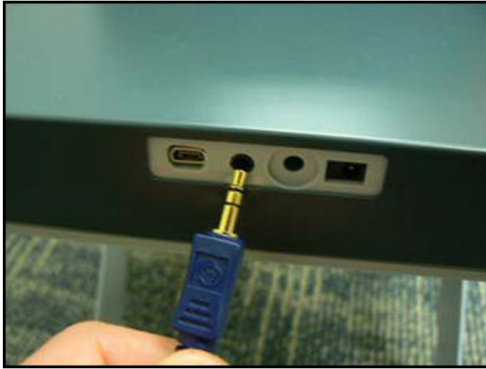
Figure 5. Plugging the Remote Trigger Cable Into the Portable Test Stand
