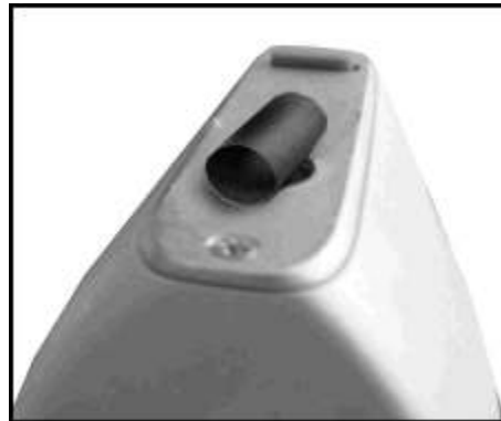
Figure 39. Incorrect Way to Measure Heat Shrink Tubing
