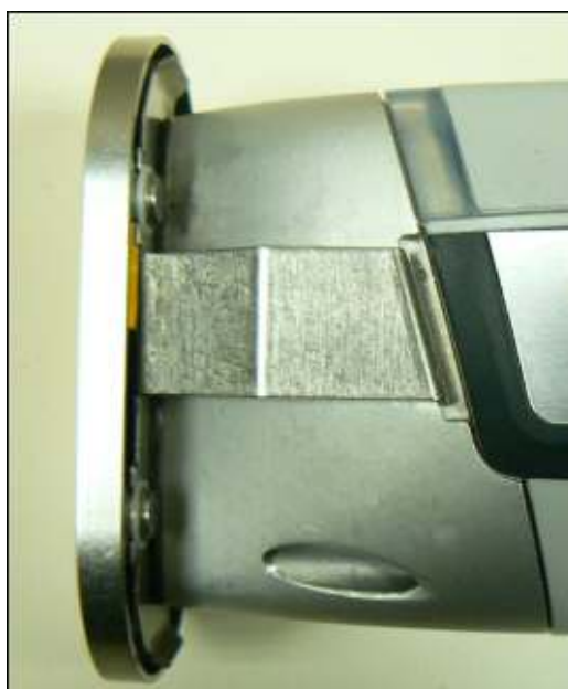
Figure 3. The In-Situ Test Guard in Place
