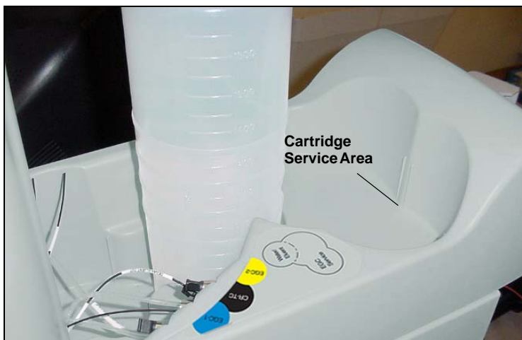
Figure 5-47. Dionex EluGen Cartridge Service Area
