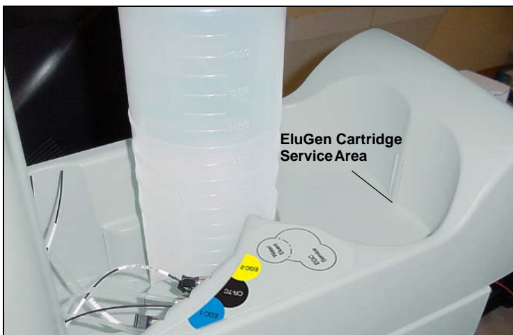
Figure 5-36. Dionex EluGen Cartridge Service Area
