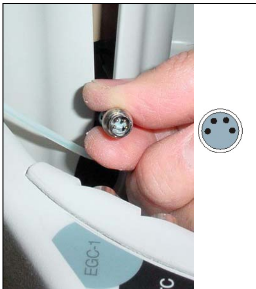
Figure 5-53. Connecting the Dionex EluGen Cartridge Cable
