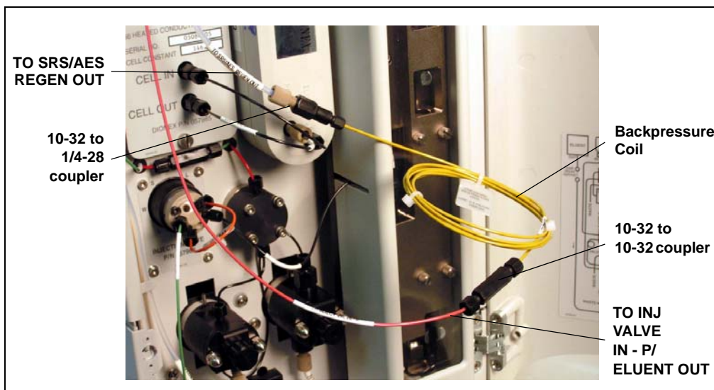
Figure 5-58. Backpressure Coil Connections for Conditioning the EPM with Carbonate/Bicarbonate Eluent
