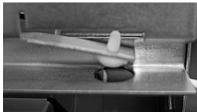
Figure 16. The canoe-clips hold the accessory in place firmly against the flame shield
