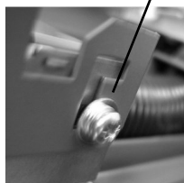
Figure 12. The support bracket in the position for Zeeman instruments
