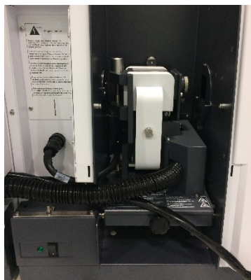
Figure 5. Power cable plugged into connector on the 280Z AA
