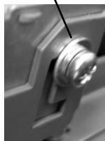
Figure 13. The support bracket in the position for D 2 instruments
