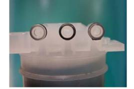
Install the SynergyPak until it is fully seated into the system ports as shown (C, D and E).
