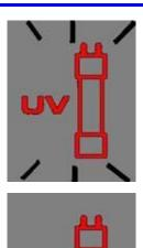
The system will prompt you to change the UV Lamp using a red UV Lamp Alarm icon. The Display will show the red UV Lamp Alarm blinking. The message is shown when the UV Timer displays 0 days. The UV Timer can be viewed in menu option CO3. The replacement of the UV Lamp involves the installation of a new UV Lamp and a manual reset of the UV Timer.
