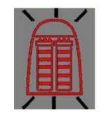
The system will prompt you to change the SynergyPak using a red Pack Alarm icon. The Display will show the red Pack Alarm blinking. The SynergyPak is changed due to either the amount of time it has been used or from the amount of water that has passed through it.
