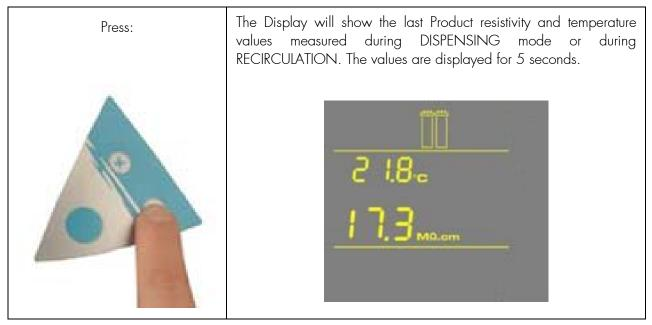
NOTE: The Product resistivity and temperature are displayed automatically during DISPENSING mode or during RECIRCULATION.
