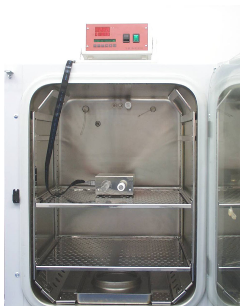
Figure 33: Measuring with CTM 01 (door is closed during measurement)
