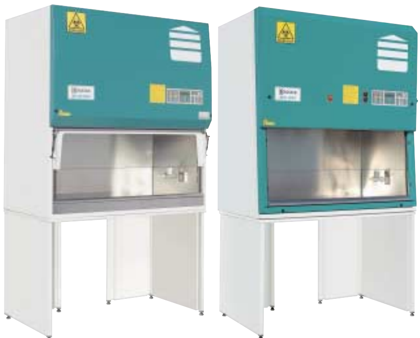
BHG cabinet features an ergonomically angled sloping-front, fitted with electrically operated vertically sliding safety-glass sash window, the framework of which is also hinged and can be opened up for easy access during cleaning and maintenance.
