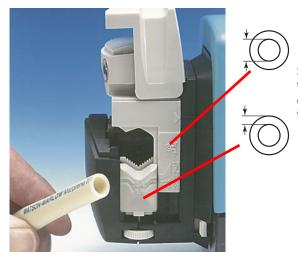
Set the tube clamps to the correct tube size. The track must be fully open. Align the scale on both sides of the pumphead.
