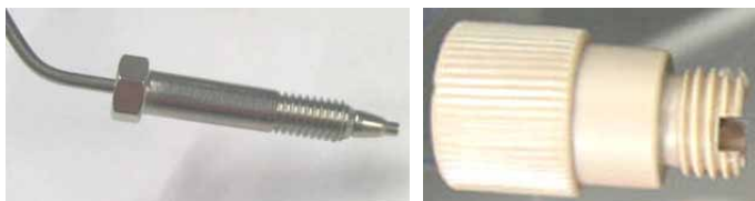
Fig. 61: Fitting for the needle end of the sample loop
