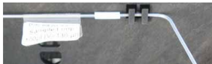
Fig. 57: Clip securing the sample loop in position
