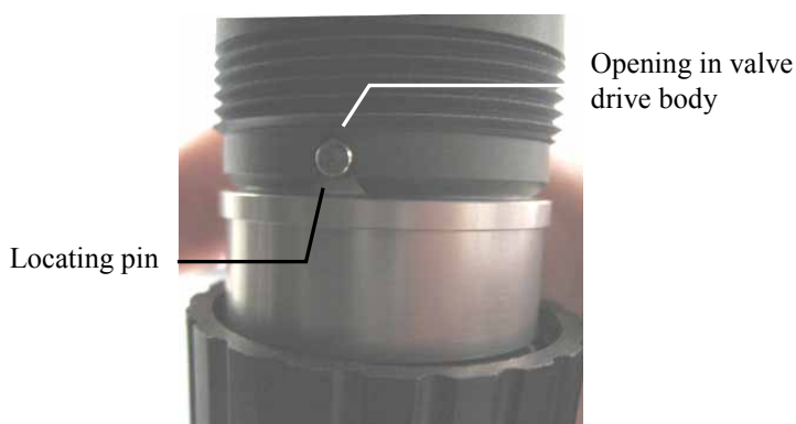
Fig. 82: Aligning the locating pin
