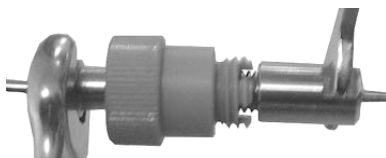
Fig. 59: Disconnecting the sample loop from the needle
