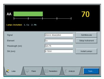
Lamp Setup page automatically sets up the instrument when using a coded Lumina lamp.
