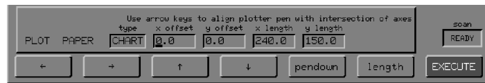
Figure 4-14 Command Line and Soft Keys for Aligning the Pen with Chart Paper
