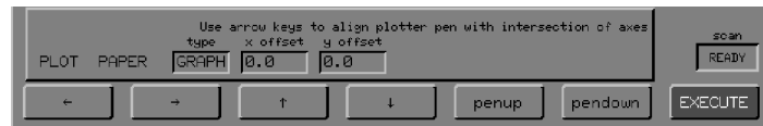
Figure 4-15 Command Line and Soft Keys for Aligning the Pen with Graph Paper
