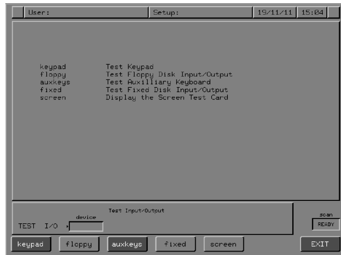
Figure 3-6 The Test I/O Screen
