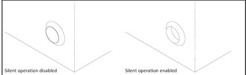
Enabling silent operation on the temperature control unit reduces the noise level by decreasing the pump capacity. For the exact position of the switch **>Change pump speed<** [114] please refer to the "Wiring diagram".  $\rightarrow$  From page 69, section **>Annex**«.
