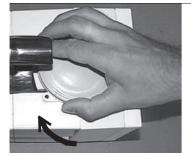
The diaphragm and the diaphragm holder can then carefully be screwed on and tightened by hand with the same force as your have needed to detache it before! Check again if there is **no gap** between diaphragm and holder after replacing the diaphragm.
