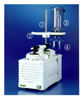
Fig. 16: VAC V-501 with secondary condenser
