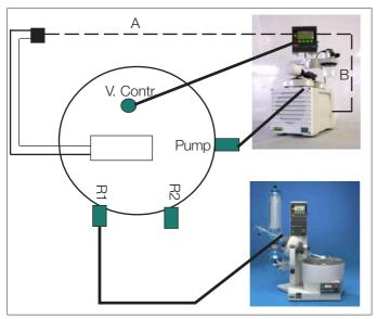
Fig. 19: Installation Vac V-502 with V-800 with Rotavapor
