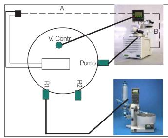
Fig. 21: Installation Vac V-503 with V-800 with Rotavapor
