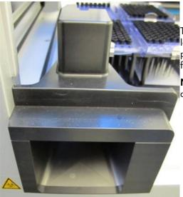
Tips used on the worktable are discarded through the tip ejector located on the left side of the QIAgility. The tip ejector is held in place by a locating block, allowing easy placement and removal for cleaning.
