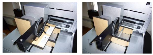
2. Move the pipettor head to the right and remove the transport lock from the worktable.
