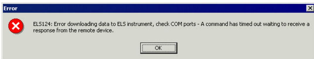
In this case, check that the Detector is connected to the PC and is switched on.
