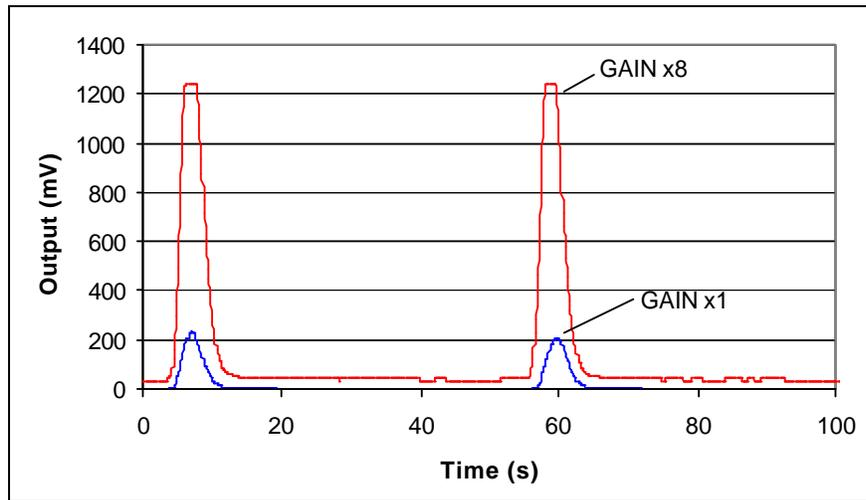
Figure 2.3.1 Example of Changing the Pmt from 1 to 8
