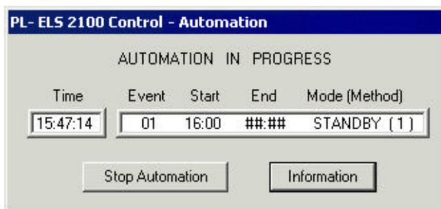
The automation procedure can be stopped at any point by selecting *Stop Automation*.
