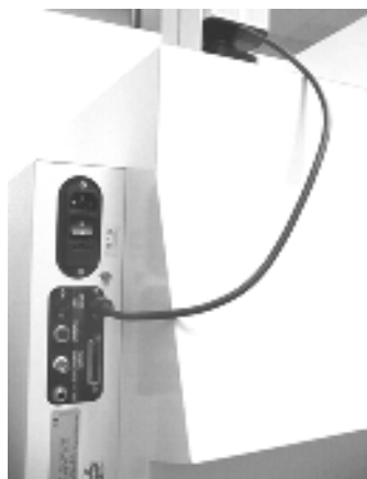
Motorized Zoom Lens control cable
