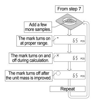
Note ACAI will not function on the unit mass entered using the keys, or digital input mode.
