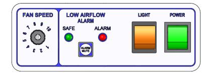
The booth is started by first operating the Green rocker switch on the control panel. The Red airflow monitor warning light will flash until the correct airflow is achieved.
