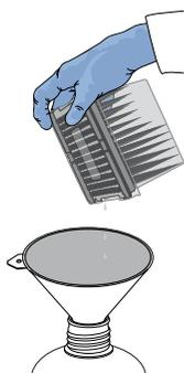
**IMPORTANT!** Do not reuse the waste pipette tip rack. Always move the empty Tip Cartridge v2 from the new tip position to the waste tip position.
