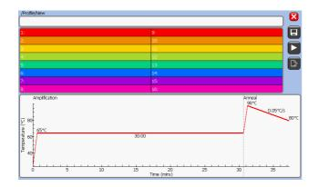
Press the 'New' button on the profile screen. Click the graph to adjust the profile by touching the appropriate temperature or time box.
