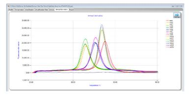
The 'Anneal Derivative' tab shows the plot of the derivative of fluorescence for each well made during the Anneal phase plotted against temperature.
