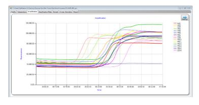
The 'Amplification' screen displays the fluorescence measurements for each well made during the Amplification phase plotted against time.
