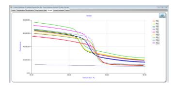
The 'Anneal' tab shows the plot of the fluorescence measurements for each well made during the Anneal phase plotted against temperature.
