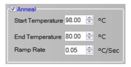
If the assay requires an anneal, check the 'Anneal' box and alter the start temperature, end temperature and cooling ramp rate. This dialogue box shows how to set an annealing curve from high to low temperatures.
