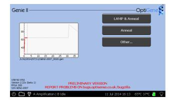
When a run is started, the main screen will display a preview of the run that is active. As the run progresses, the grey line showing the profile will turn red.
