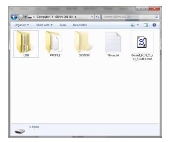
To install the updates, connect Genie® II to a computer. Navigate to 'My Computer' and open the Genie® II drive. The drive is named with the instrument serial number, e.g. GEN2-2001. Copy and paste (or drag) the firmware or FPGA software files onto the Genie® II drive.
