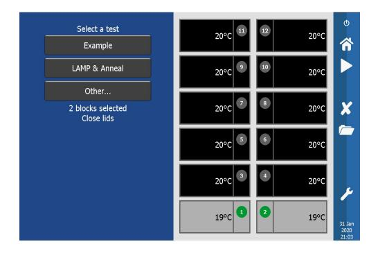
Once all the blocks are selected the next step is to select a test. Buttons can be assigned (in the Settings menu) to profiles and are shown on the left. Alternatively, touch 'Other...' to create a new profile, or open another saved profile. The numbers of blocks selected are listed, along with the reminder to close the lids. A run cannot be started until all the lids are closed.
