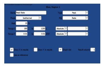
The points at which the criteria are met are marked by a dot on the graph line.
