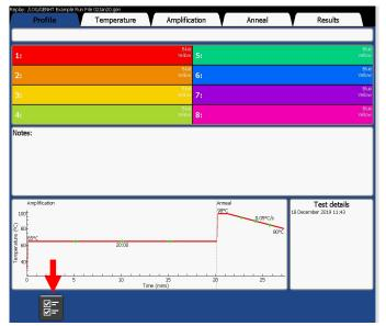
Pressing this button on the profile screen will allow the user to change the parameters for result calling for the profile. All the parameters are stored within the profile and the run file.
