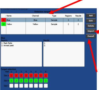
This screen shows an overview of the 'Detection targets', showing the number of regions of interest, the number of results, and which targets are assigned to which well. From here new targets can be added, imported from other runs or profiles, edited or deleted.
