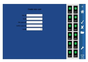
To create a new user, click on the Add User button (shown), and then enter the details for the user and select an access level. Press the tick to save, or the cross to cancel (in the menu bar).
