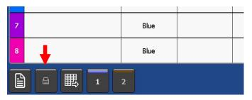
Pressing the button shown on the results table will print the table onto a label if the correct printer is attached to the Genie® instrument via the USB ports on the front of the instrument.
