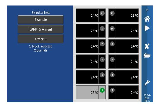
**TIP!** By opening a lid or by pressing a block will result in the block automatically being selected.
