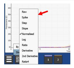
Selecting 'Show plot' will produce a second menu to select which plot to display on the screen depending on which signal processing step is wanting to be viewed. These are explained below and further in Chapter 6.
