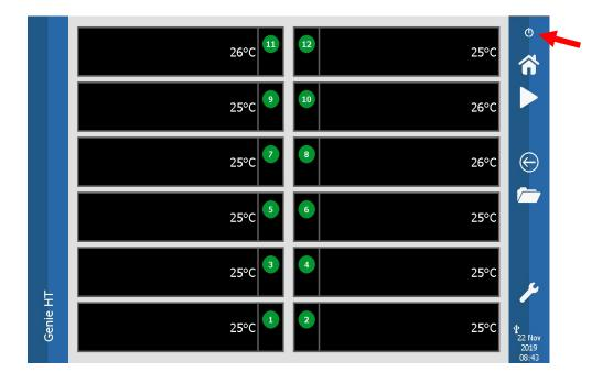
Note: If this button is pressed during a run, Genie® HT will not enter standby.
