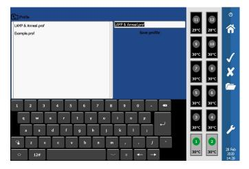
Pressing the save icon will save the profile. Name the profile, press the tick button and it will be saved within the 'PROFILE' directory in the on-board memory allowing it to be loaded for future runs.
