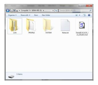
To install the updates, connect Genie® HT to a computer. Navigate to 'My Computer' and open the Genie® HT drive. The drive is named with the instrument serial number, e.g. GEN3-1001. Copy and paste (or drag) the firmware or FPGA software files onto the Genie® HT drive.
