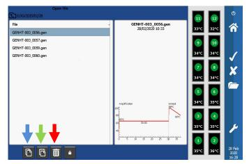
The default filename for the each run is the instrument serial number followed by a sequential number.
