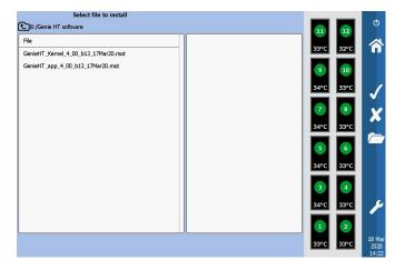
Touch on the file, and touch the tick button. The Genie® HT will then install the updated software and restart the instrument. Please wait for it to finish before trying to do anything else.
