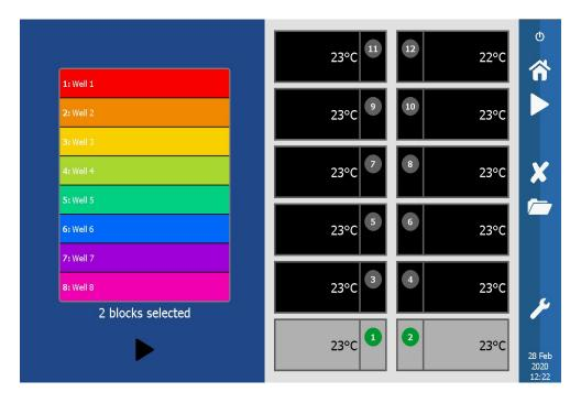
Once a test is selected, the well names are shown along with the number of blocks selected and, once the lids are closed, a play button. Pressing this will start the run. Touching on the well names will allow editing of the profile, which is explained later.
