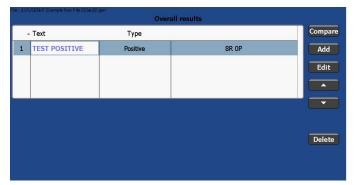
This screen shows the defined overall results. Result definitions are tested in order. The first matching result is displayed. This order can be changed using the up and down arrow buttons.
